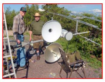
WA3RLT and WA3GFZ attaching the 10GHz feed
